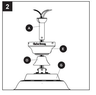
Slide the downrod (A) into the yoke of the motor assembly (G), align the holes, then re-install the downrod clip (C) and downrod pin (B). Secure with set screws (Q).
