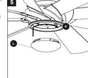
5. Lift the glass bowl (L) over the light kit (K) and turn in a clockwise direction until it is secure.
