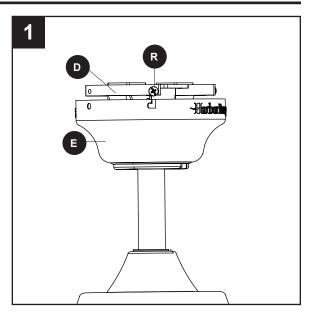
Secure the canopy (E) with the mounting bracket screws (R) previously removed (Step 4, page 8). Tighten all mounting bracket screws (R) securely.
