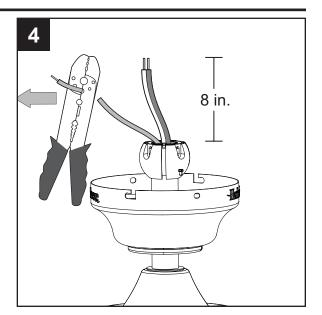
If you decided to cut back the lead wire in Step 4, strip 1/2 in. of insulation from the end of the white wire. Twist the stripped ends of each strand of wire within the insulation with pliers (not included). Repeat this step for black and green wires.
