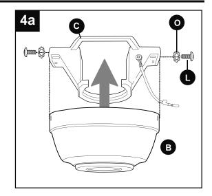
4b. Secure mounting bracket (C) to outlet box (not included) using screws, spring washers and flat washers provided with the outlet box.
