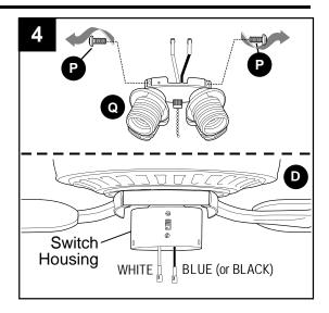
Connect WHITE wire from switch housing to WHITE wire from light kit fitter (Q). Connect BLUE (or BLACK) wire from switch housing to BLACK wire from light kit fitter (Q). Make sure molex connections are secure.
