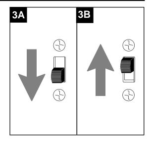
3C. **IMPORTANT**: Reverse switch must be set either *completely UP* or *completely DOWN* for fan to function. If the reverse switch is set in the *middle* position, fan will not operate.
