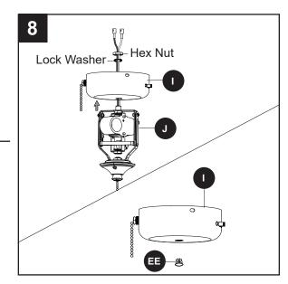
9. Remove the three switch housing screws (X) from the fitter plate (H). Then, attach the switch housing (I) to the fitter plate (H) using the switch housing screws (X).
