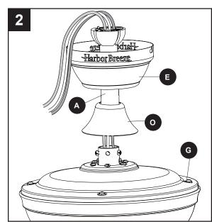
3. Slide the downrod (A) into the yoke of the motor assembly (G), align the holes, then re-install the downrod clip (C) and downrod pin (B). Secure with set screws (W).
