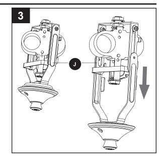
4. Once maintenance has been performed, simply lift the glass bowl (N) up to its original position. The light kit fitter (J) is secure once it clicks into place.
