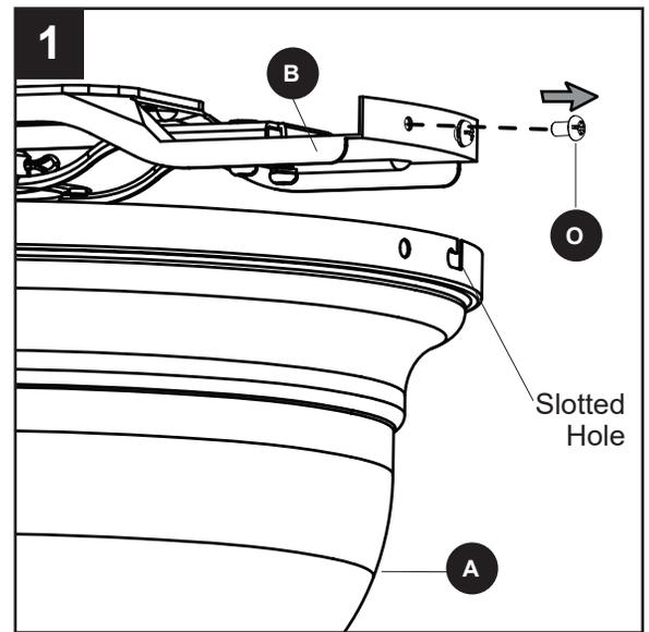
2. Slide the motor housing (A) over the motor (E), aligning the slotted holes in the motor housing (A) with the loosened motor housing screws (O) in the upper mounting bracket (B). Twist the motor housing (A) clockwise to lock. Then re-insert the two previously removed motor housing screws (O) and securely tighten all screws.
