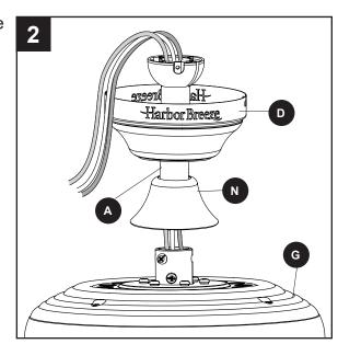
3. Slide the downrod (A) into the yoke of the motor assembly (G), align the holes, then re-install the downrod clip (C) and downrod pin (B). Secure with set screws (T).
