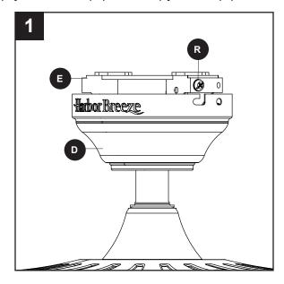
2. Secure the canopy (D) with the mounting bracket screws (R) previously removed (Step 4, page 8). Tighten all mounting bracket screws (R) securely.
