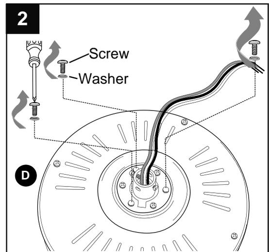
3. Pull wires up through hole in the middle of the canopy (B) and attach canopy (B) to motor housing (D) using the three previously removed screws and lock washers.
