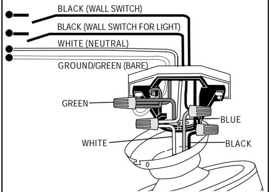
**NOTE:** BLACK wire is hot power for fan. BLUE wire is hot power for light kit. WHITE wire is common for fan and light kit. GREEN or BARE wire is ground.
