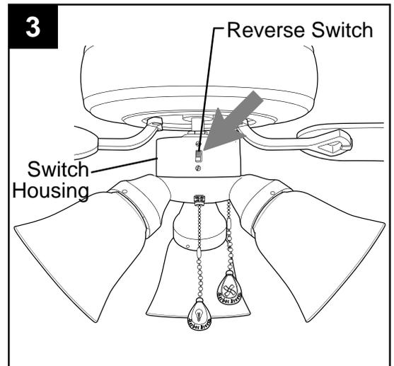
3A. In **warmer** weather, setting the reverse switch in the *DOWN* position will result in downward airflow creating a wind chill effect.
