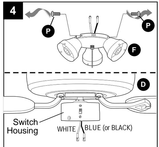
5. Connect WHITE wire from switch housing to WHITE wire from light kit fitter (F). Connect BLUE (or BLACK) wire from switch housing to BLACK wire from light kit fitter (F). Make sure molex connections are secure.
