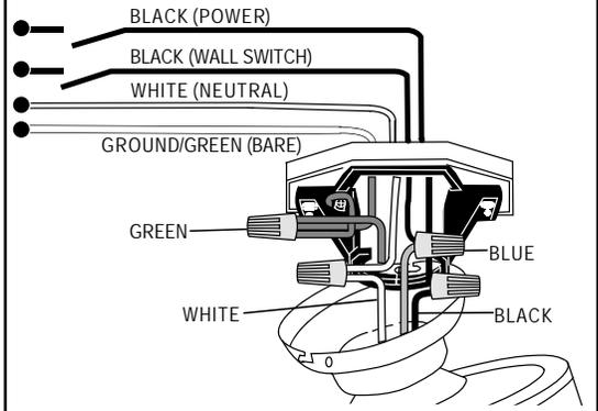
**1c. FAN AND LIGHT CONTROLLED BY TWO WALL SWITCHES:** Connect BLACK wire from fan to BLACK (or RED) wire from the independent wall switch for the fan. Connect BLUE wire from fan to the BLACK (or RED) wire from the other independent wall switch for the light. Connect WHITE wire from fan to WHITE wire from ceiling. Connect GROUND (GREEN) wires from downrod (A) and mounting bracket (C) to BARE/GREEN wire from ceiling.
