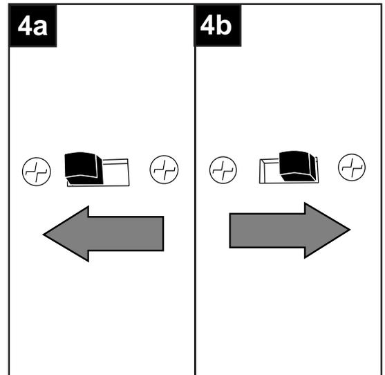
4c. **IMPORTANT:** Reverse switch must be set either **completely** LEFT or **completely** RIGHT for fan to function. If the reverse switch is set in the middle position, fan will not operate.
