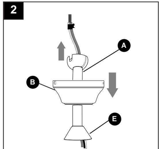
3. Slip downrod (A) into yoke, align holes and re-install pin (L) and clip (M). Tighten set screws and then tighten nuts. Slide yoke cover (E) down until it rests on top of motor housing (D).
